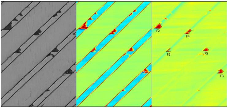
Three views of a small caliber barrel. From Left: LaserVideo™ Image, Laser Profile Data, Automatic Feature Detection
